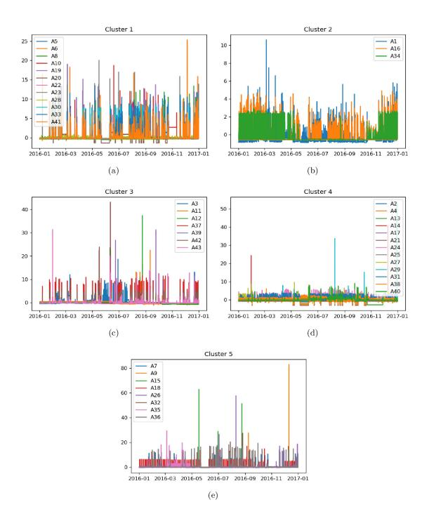
Figure 4.6: Static Time-series clustering of 43 appliances into 5 clusters. (a) Appliances group of Cluster 1. (b) Appliances group of Cluster 2. (c) Appliances group of Cluster 3. (d) Appliances group of Cluster 4. (e) Appliances group of cluster 5. using k-shape algorithm. The shape of different time series in a cluster shows strong similarity.
