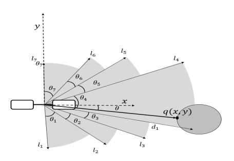
Figure 3: Obstacle effective range and turning radius for avoiding the obstacles.
