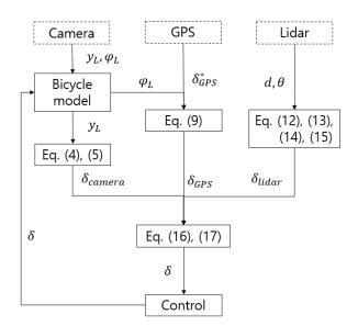
Figure 4: System model of bicycle robot control.
