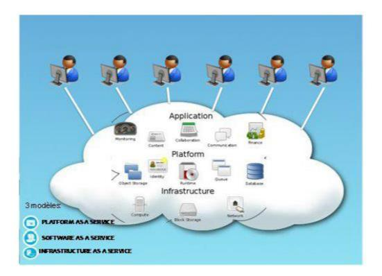
Figure 2: The 3 cloud computing models.
