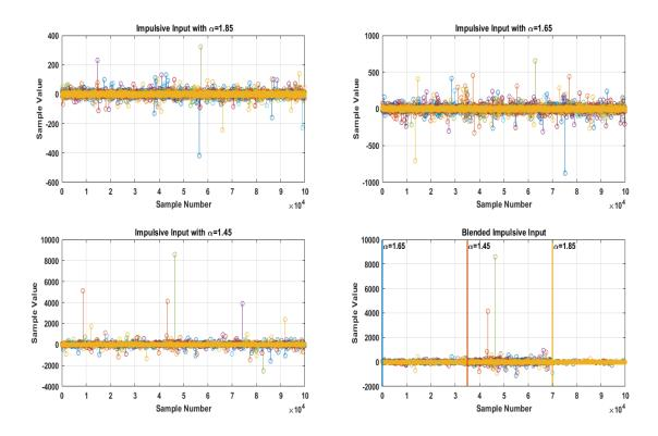
**Figure 10:** (a) Moderate impulsive input ( $\alpha$ =1.85), (b) High impulsive input ( $\alpha$ =1.65), (c) Very High impulsive input ( $\alpha$ =1.65), (d) Blended impulsive input.
