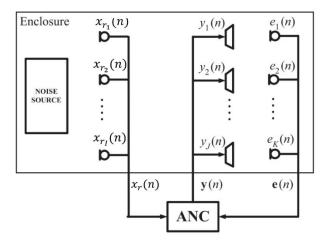
**Figure 3:** Structure of  $I \times J \times K$  MC ANC system.
