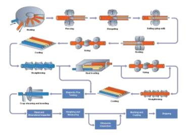
Figure 2. Plug Process (https://www.wermac.org/pipes/pipemaking.html)
