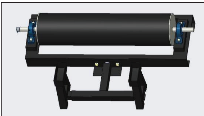
Figure 2 – An overview of the proposed inertial dynamometer
