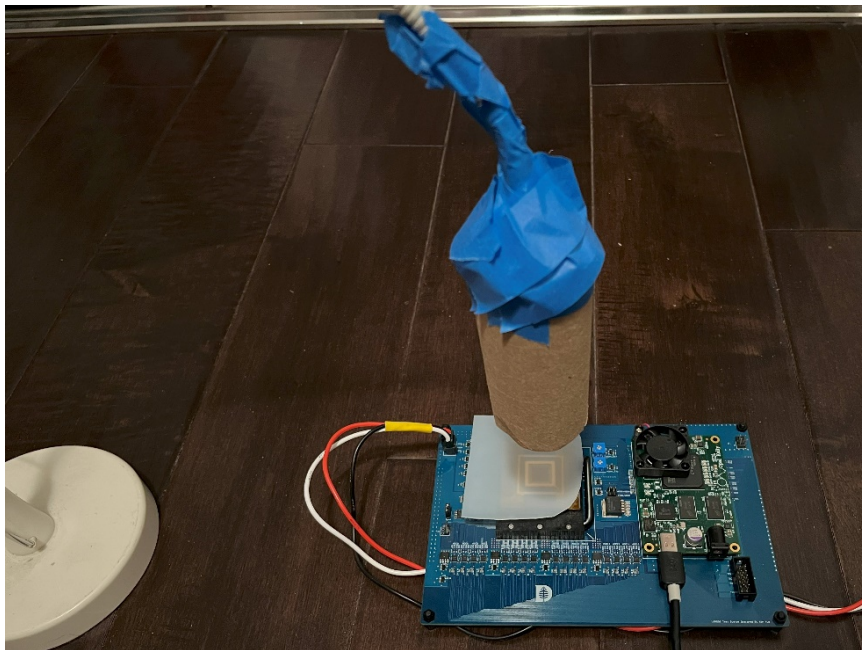
Home lab setup with integrating cylinder, diffusion lens and desk lamp
