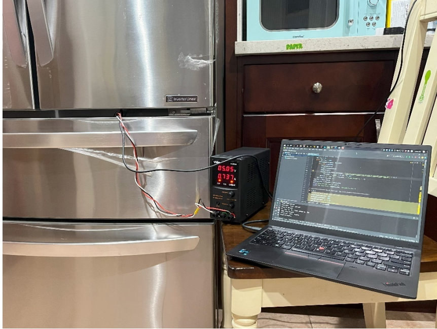
Home lab setup for dark current measurement (test system in the refrigerator)
