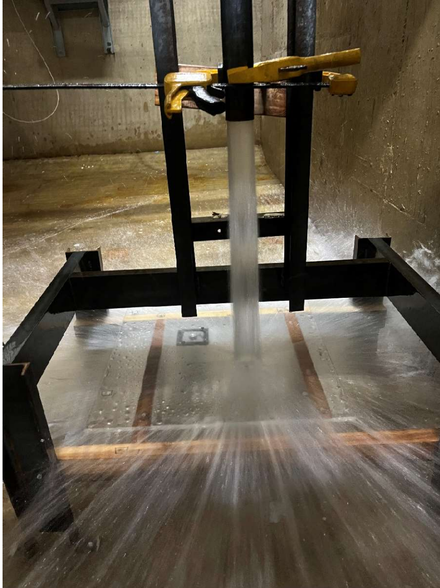
Figure D-4 – Falling jet approximately 22 fps and 2-foot fall height.
