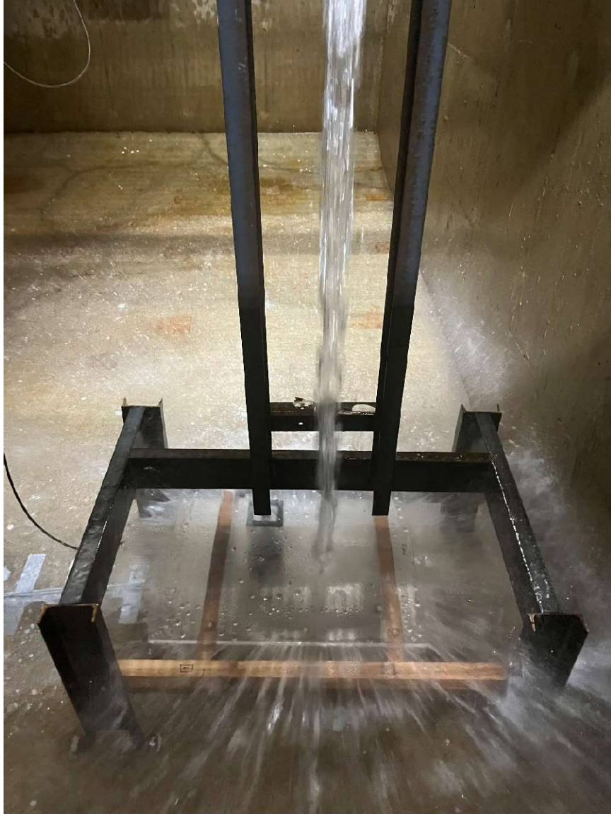
Figure D-12 – Falling jet at approximately 14 fps and 10-foot fall height (lower section).
