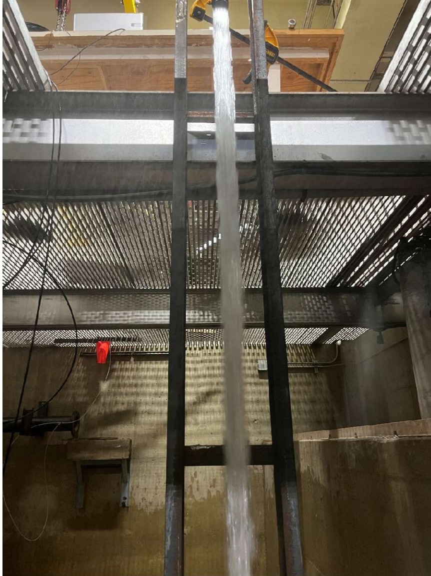
Figure D-13 – Falling jet at approximately 19 fps and 10-foot fall height (upper section).
