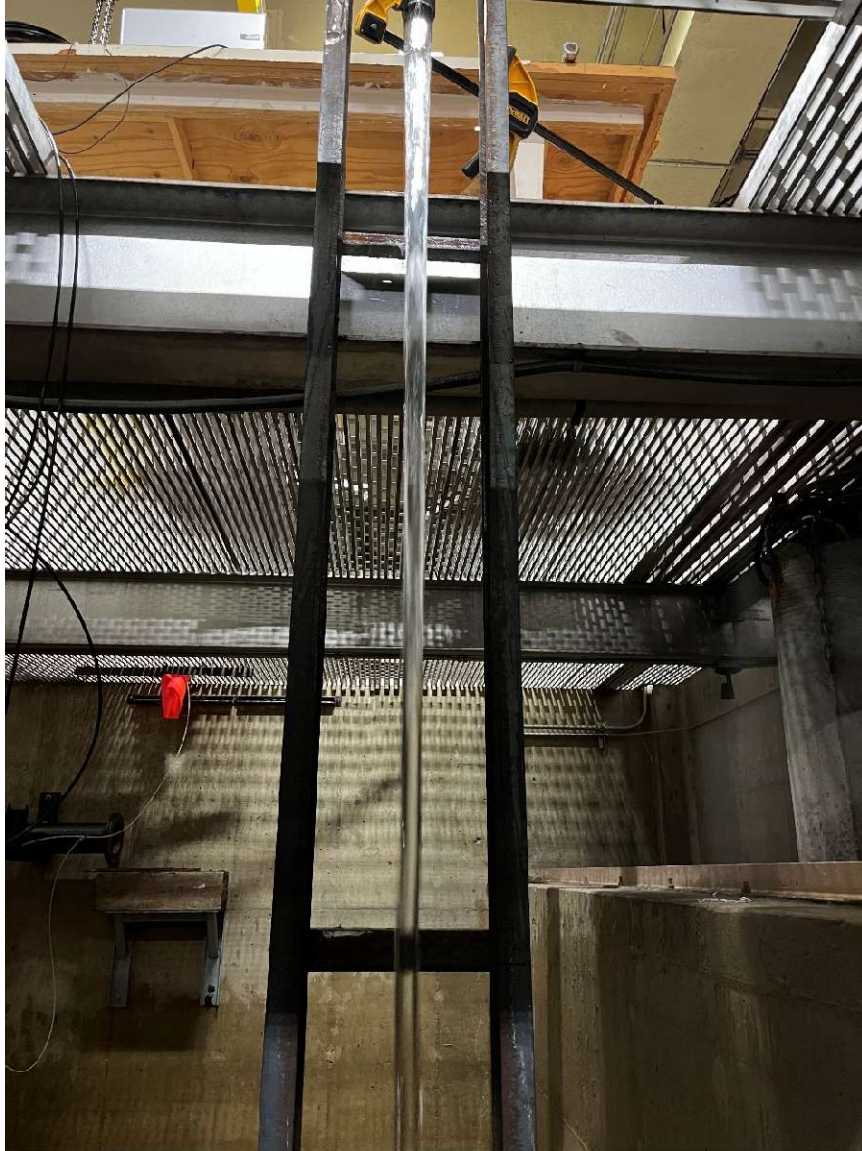
Figure D-9 – Falling jet at approximately 5 fps and 10-foot fall height (upper section).
