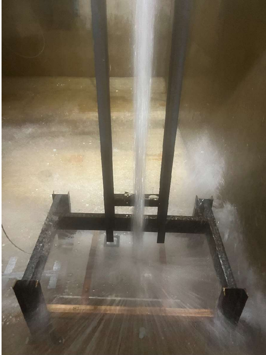
Figure D-16 – Falling jet at approximately 22 fps and 10-foot fall height (lower section).
