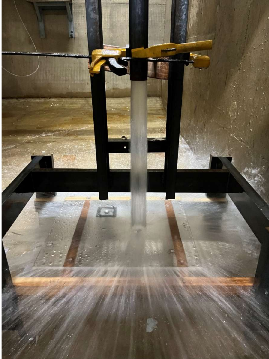
Figure D-3 – Falling jet approximately 19 fps and 2-foot fall height.
