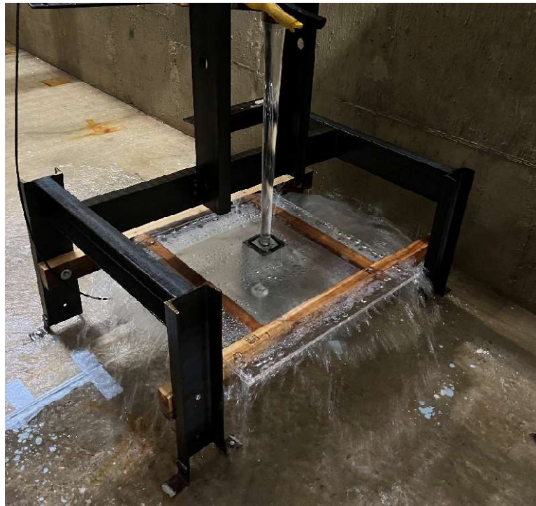
Figure 4 – Plexiglass platform for testing instrumentation.
