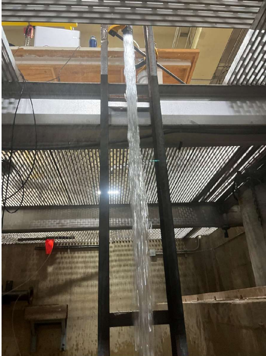
Figure D-11 – Falling jet at approximately 14 fps and 10-foot fall height (upper section).
