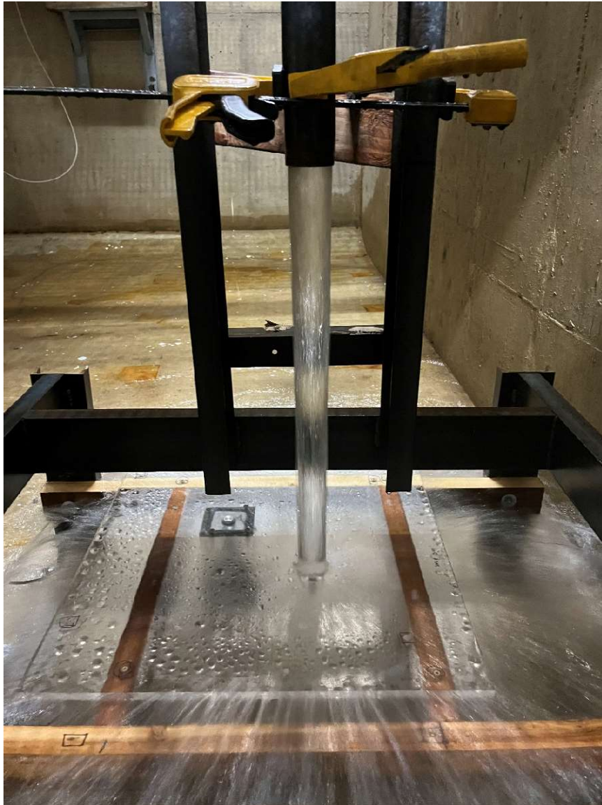
Figure D-2 – Falling jet approximately 14 fps and 2-foot fall height.
