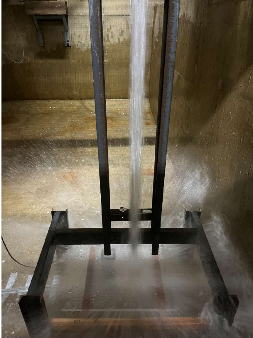
Figure D-14 – Falling jet at approximately 19 fps and 10-foot fall height (lower section).
