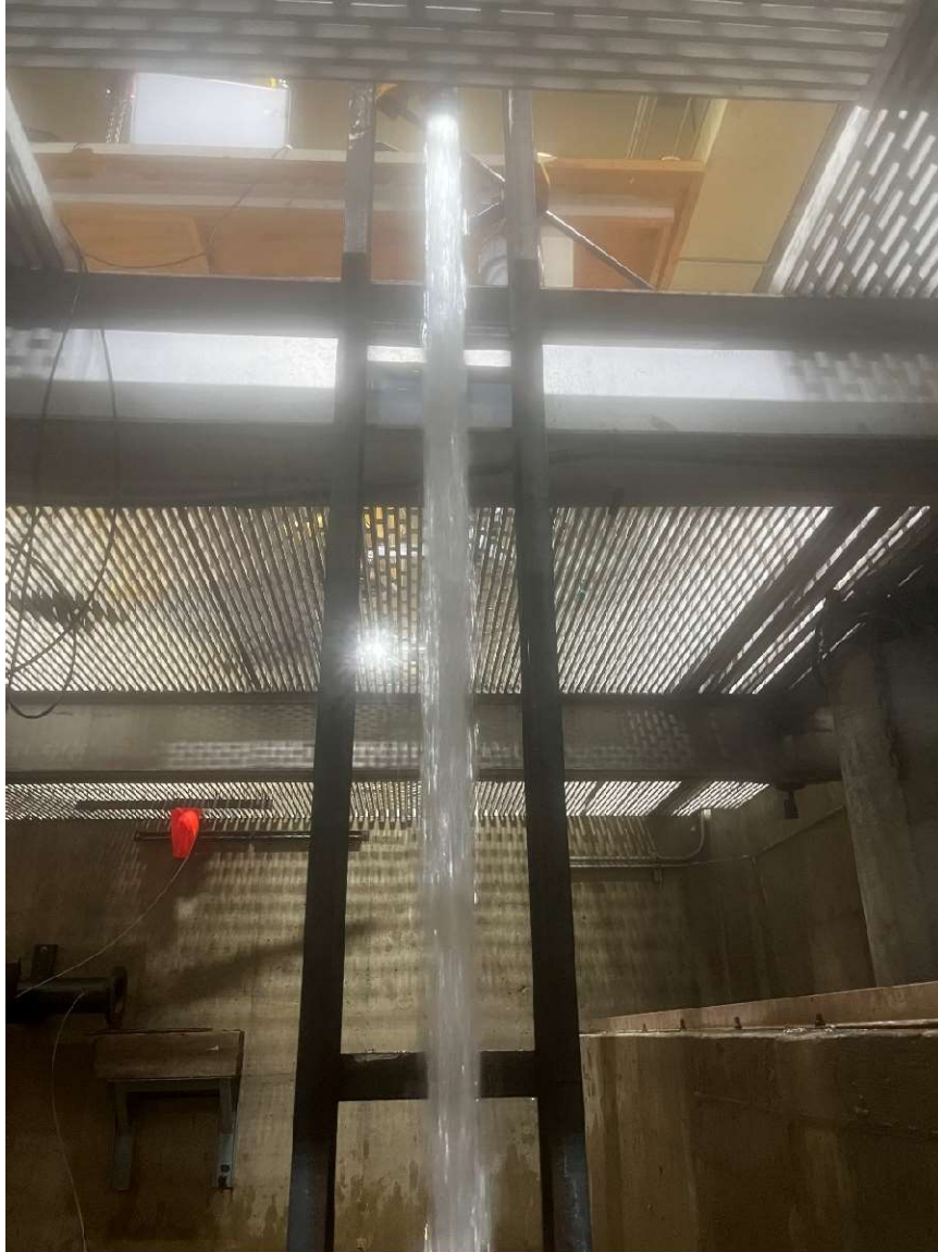
Figure D-15 – Falling jet at approximately 22 fps and 10-foot fall height (upper section).
