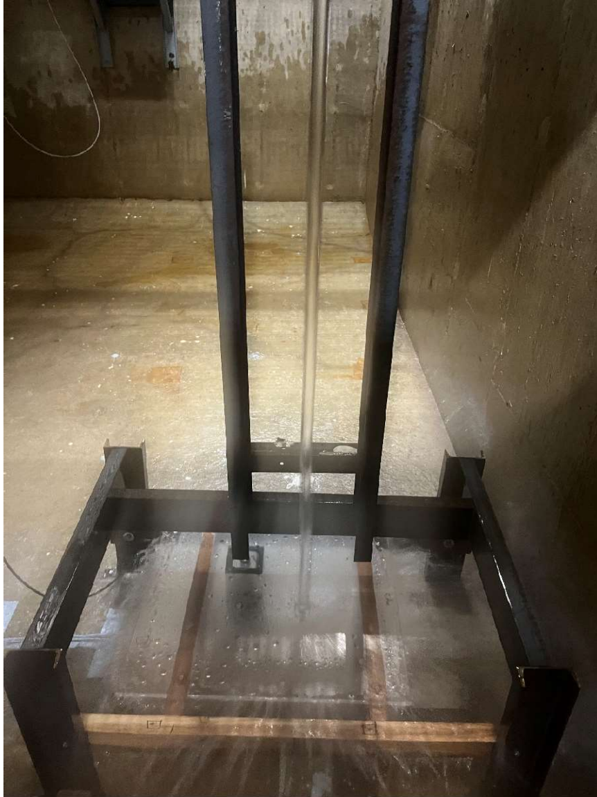
Figure D-10 – Falling jet at approximately 5 fps and 10-foot fall height (lower section).
