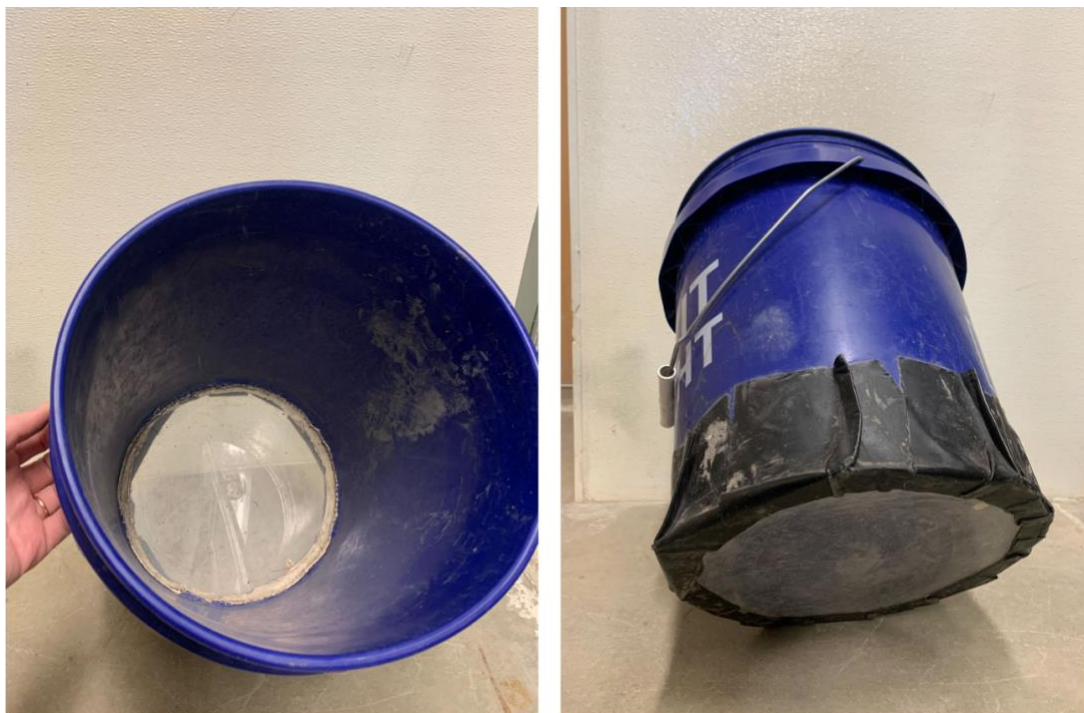
Figure S3.3. Bathyscope used to improve visibility to visually assess percent cover.
