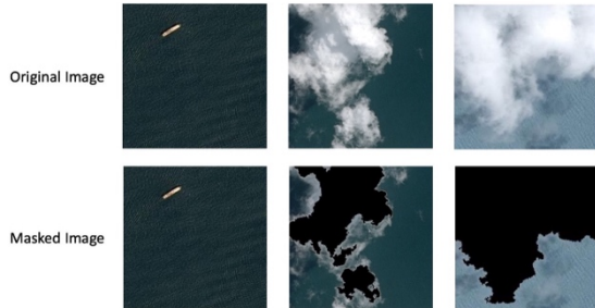
Figure 3: Clouds are masked with full black #00000000, allowing greater compression of the image.
