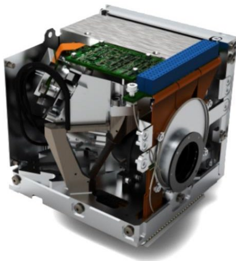
Figure 2: A Render of the CubeCAT Lasercom Terminal, Fitting in a 1U Standard Volume
