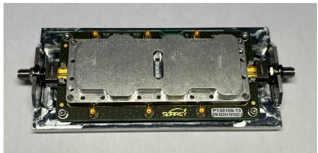
Figure 6: Lunar Pathfinder S-band EQM LNA under assembly at SSTL facilities
