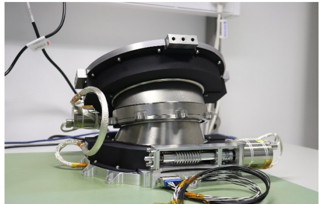
Figure 5: Lunar Pathfinder S-band antenna APM EQM on the test bench
