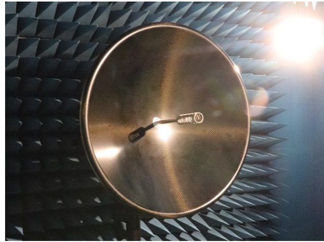
Figure 4: Lunar Pathfinder S-band antenna EQM in SSTL anechoic chamber undergoing RF testing
