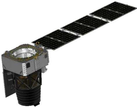
Figure 3: Rendering of BCT Saturn-class ESPA Grande vehicle with Pandora
