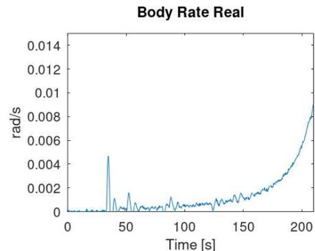
**Figure 8: LICIACube body rate [rad/s] Main rotation axis**
