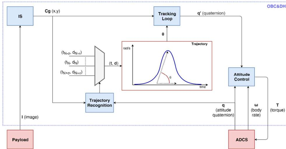
**Figure 3: Autonomous Attitude Control System functional diagram**
