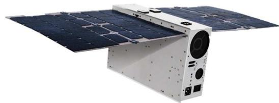
**Figure 1: LICIACube deployed configuration**
