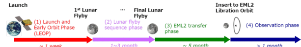
Figure 3: Overview of EQUULEUS operation phase: the period of each phase is just an example. 3
