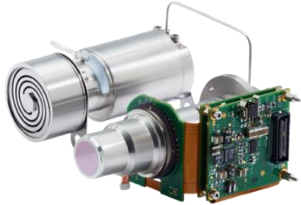
640x512px 12b 120Hz, 80K, SWIR Imager (Image: AIM)
