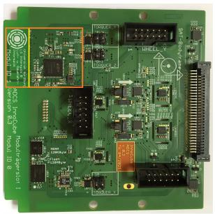
Figure 4: ADCS Board (SKITH marked orange)
