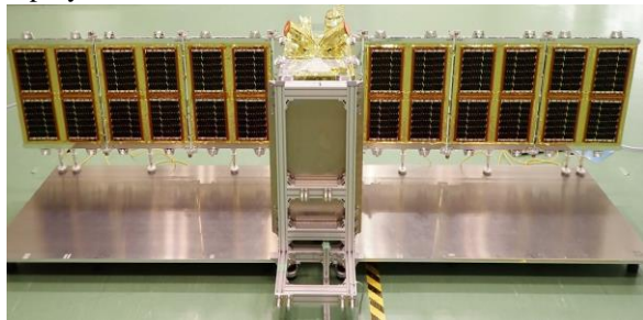
Fig. 1. Outlook of Micro-X-SAR satellite with solar cell sheets on back side of deployed antenna panels.
