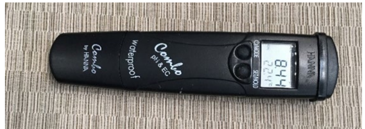
Figure 1. Example of a Handheld Water Electrical Conductivity Meter
