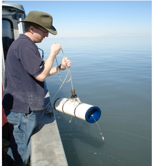
Photo 1 —Water sample collection with a Van Dorn sampling bottle.
