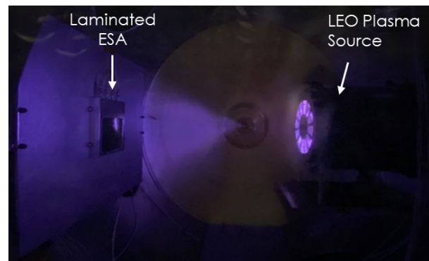
Figure 6. Photograph of the laminated collimator and ESA front-end during testing against the LEO plasma source.
