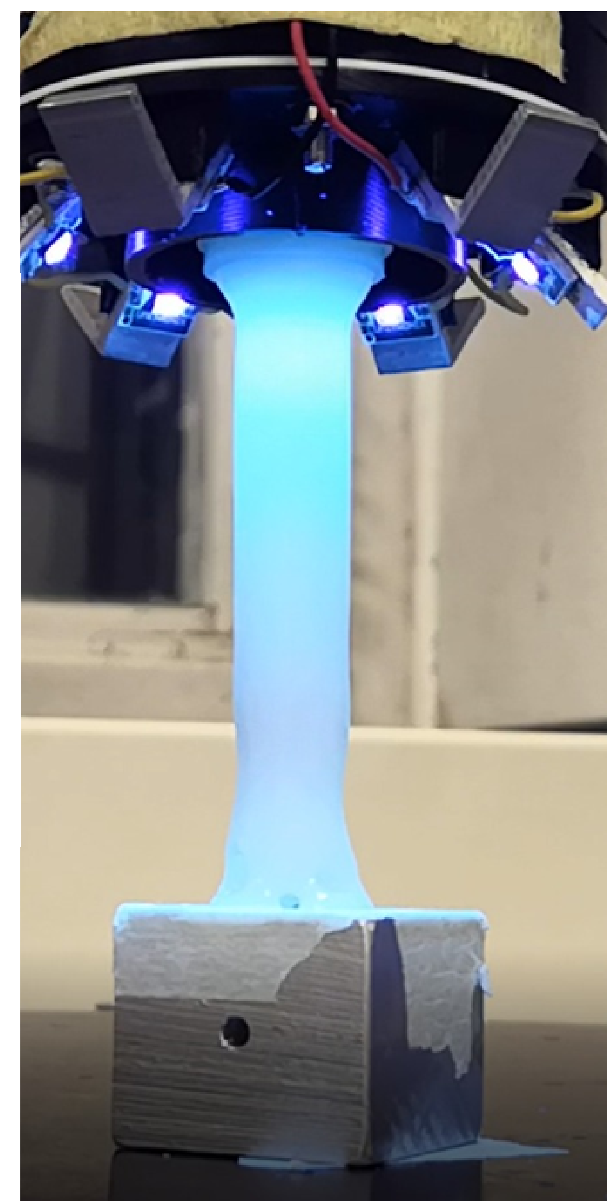
Tube nozzle during extrusion and curing
