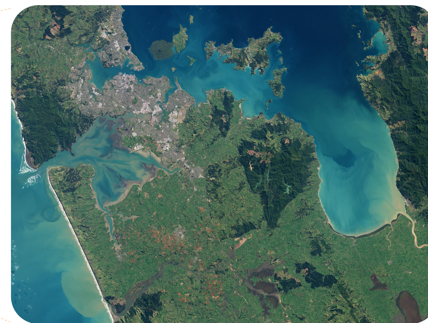
Figure 2.: Coastal water imaged by Landsat-7/ETM in March 2002. Note, however, that the spatial resolution of the image is 30m at best and the satellite revisit time is 16 days. Consequently, acute, dynamic events are poorly monitored and will have only limited value to decision makers.
