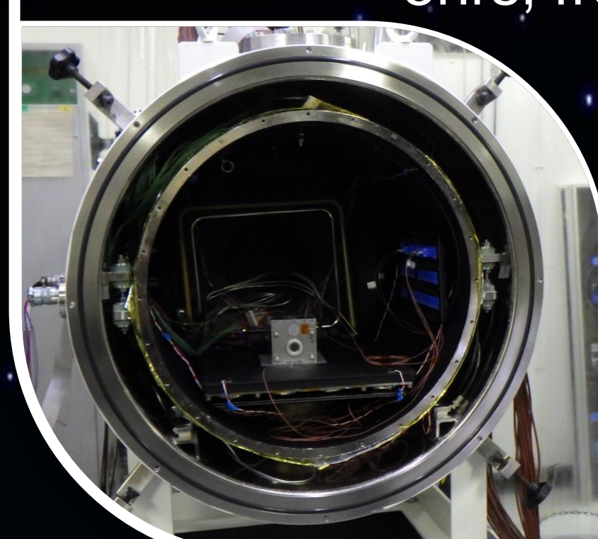
Figure 5 : Picture of the thruster in the TVAC chamber at Nagoya University
