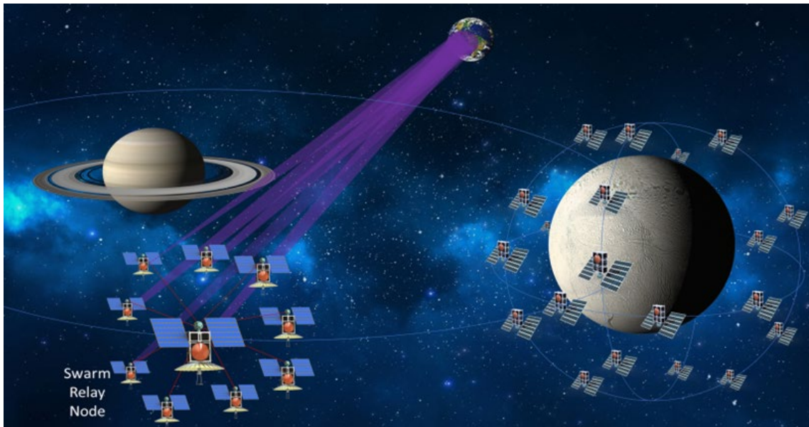
Figure 11. Notional Communication Architecture of Constellation to Relay to Earth ISL with Swarms of Spacecraft
