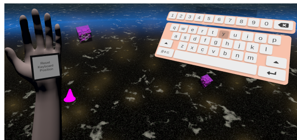
Figure 7: Dynamic keyboard with cube anchorable object next to hand representation with recenter button
