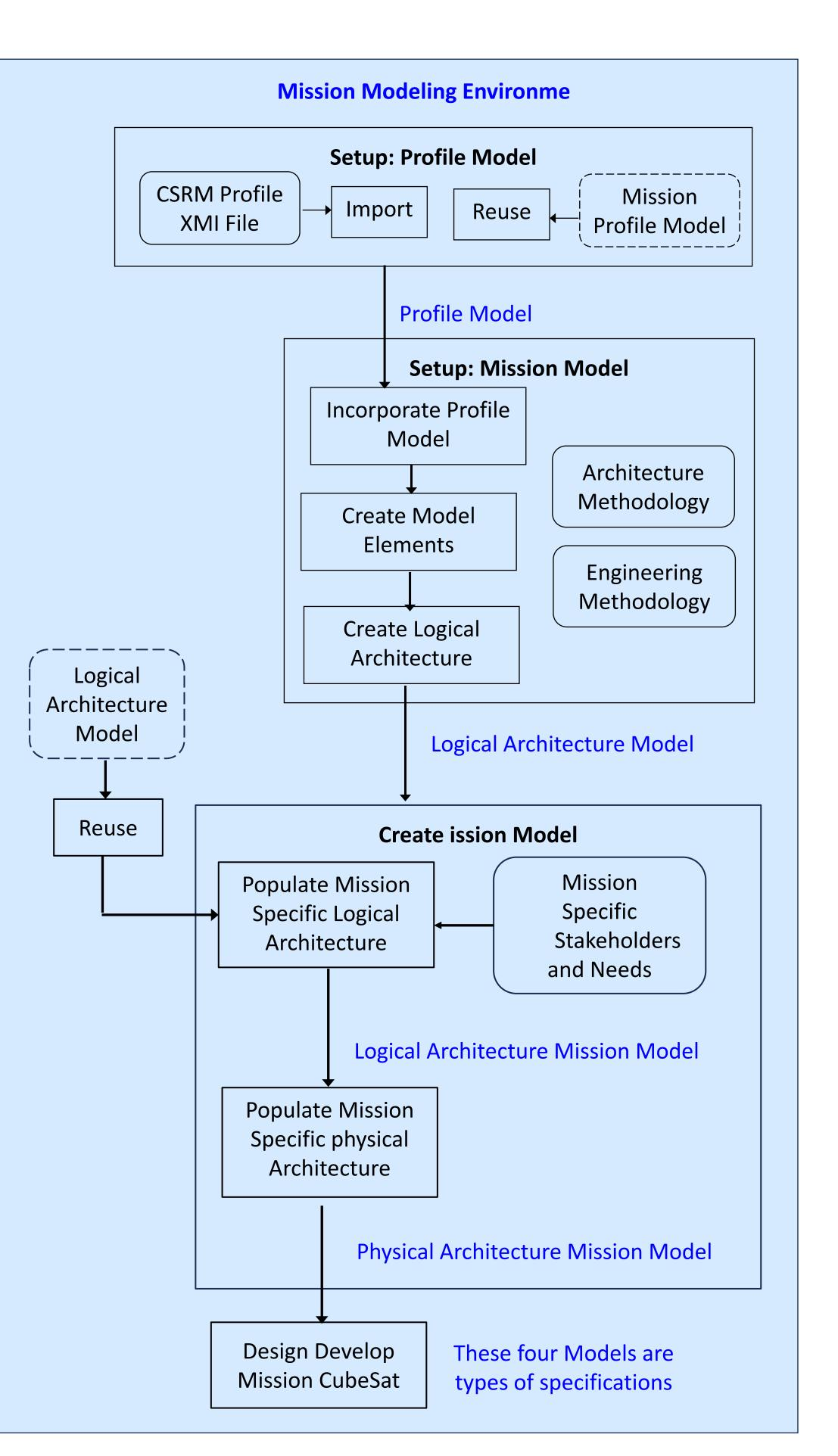
The CSRM Profile contains stereotypes that provides the building blocs for creating CSRM elements which provides he building blocks for creating the CSRM logical architecture
