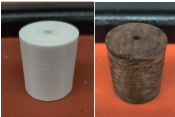
Figure 12: ABS Fuel Grain Before (left) and After (right) Catalyst Infusion
