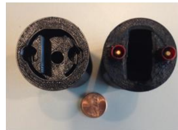
Figure 3. 3D Printed Fuel Grain with ESC-Terminated Electrodes.
