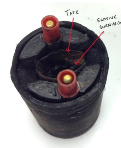
Figure 16: CatGrain and Spark Cap with Ceramic Tape
