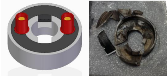
Figure 15: Boron-Nitride-Insulated Spark Cap Design (left) and Fracturing Post-Burn (right)
