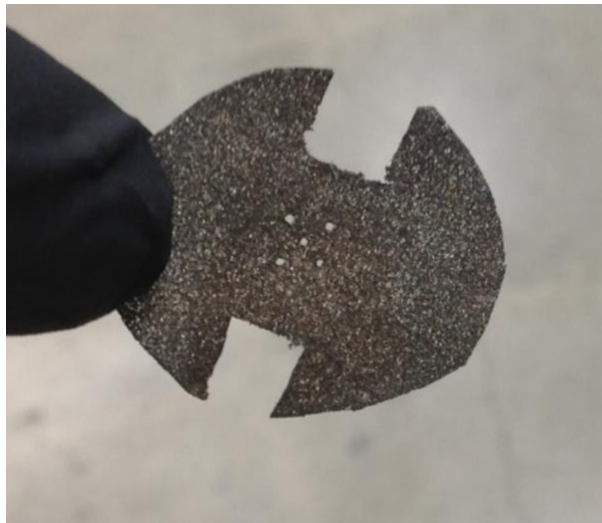
Figure 19: Nickel Foam with MnO 2 and Drilled Pass-Through Holes
