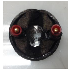
Figure 21: Burned Out Nickel Foam
