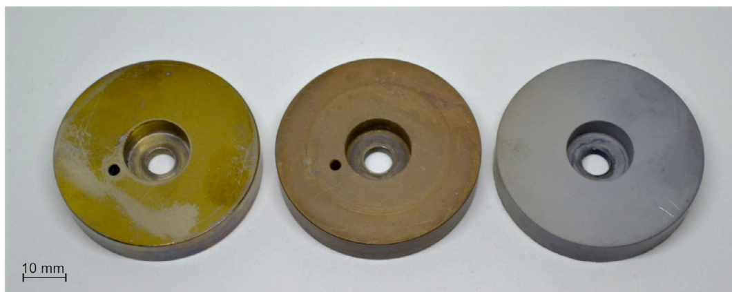
Figure 12. Ti–6Al–4V discs after ball-on-disc tests at 1000 °C in different atmospheres—from left to right—silane-doped argon, air, and argon (Photograph provided by Selina Raugel).
