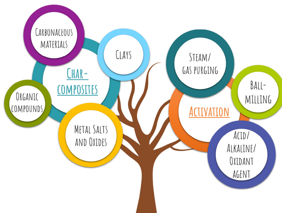
Figure 10. Chemical and physical methods of biochar and hydrochar modification.
