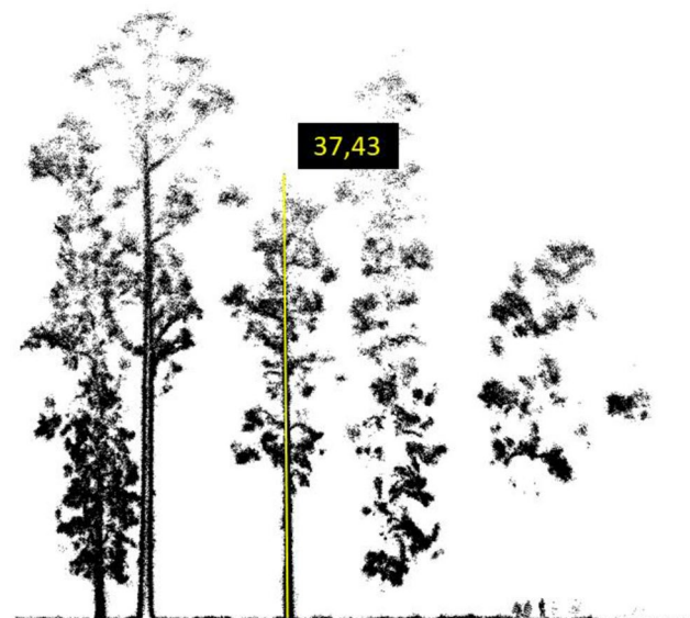
Fig. 5 Example of a height measurement made directly in a vertical slice of the PLS (portable laser scanner) point cloud
