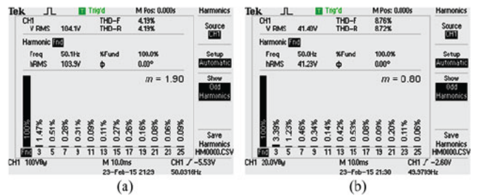
Fig. 9. Low-order harmonics of the output voltage V_s^a with CME-SVPWM. (a) m = 1.90 and (b) m = 0.80 .
