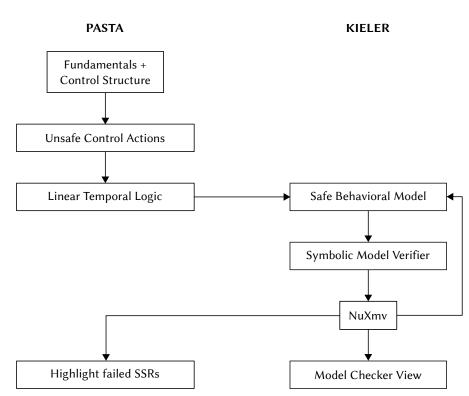
Figure 8: The workflow for model checking with PASTA.
