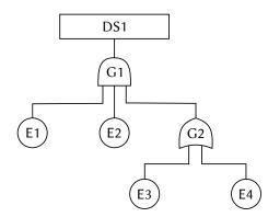
Figure 9: An example Fault Tree.
