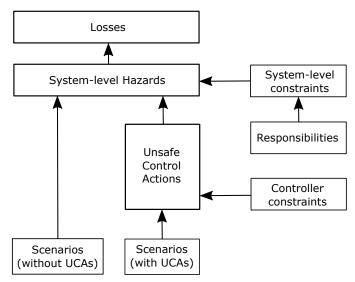
Figure 1: The STPA aspects and their connections as visualized by Leveson et al. [LT18]. A component belonging to an aspect that is the origin of an edge must reference a component belonging to the target aspect of this edge.
