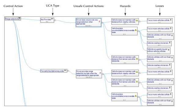
Figure 2: An extract of an example diagram in SAHRA [KRR16].
