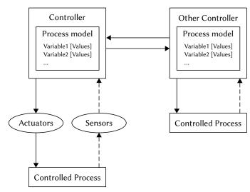
Figure 7: The planned visualization of the control structure in PASTA. The nodes represent system components while the edges represent communication between them.
