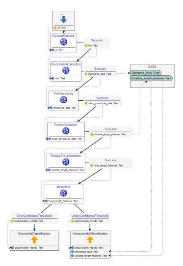
Figure 5: Top-level process model of the HIPPP system
