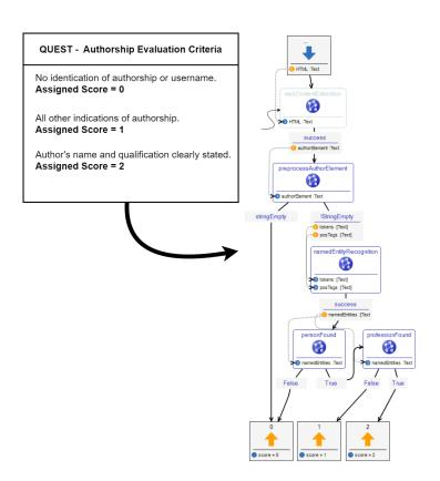
Figure 7: An example in DIME of how the QUEST authorship evaluation criteria were translated to AI and computational methods in order to automate the evaluation.
