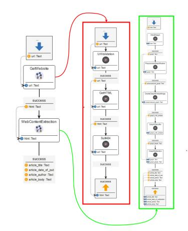
Figure 6: Hierarchical process SIBs for Website Retrieval and Web Content Extraction.
