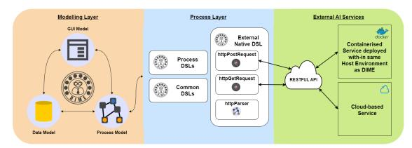
Figure 1: Overview of the DIME architecture for the LCNC AI Web App development platform
