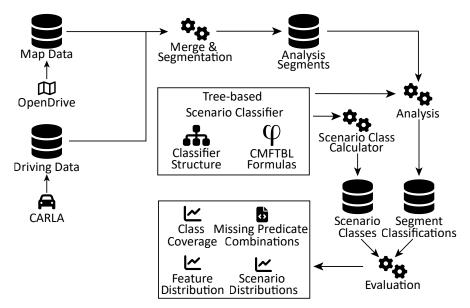
Figure 1: Overview of the tool pipeline for analyzing the coverage of test scenario sets<sup>4</sup>
