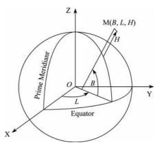
Figure 1 Definition of the geodetic system.
