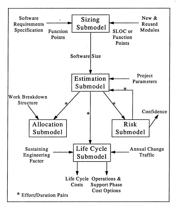
Figure 1. <u>SoftCost-R</u> Submodel Architecture
