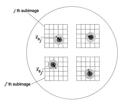
Figure 5. Wave front sensor image with compact spots overlayed on the detector pixel arrays.
