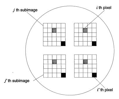
Figure 4. Pixel and subimage labeling system for the wave front sensor image. Note how the pixels labeled by  $\vec{x}_i$  and  $\vec{x}_{i'}$  are in the same relative positions in all of the subimages.
