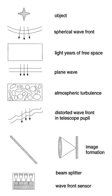
Figure 2. Wave front distortion, wave front sensing, and imaging processes
