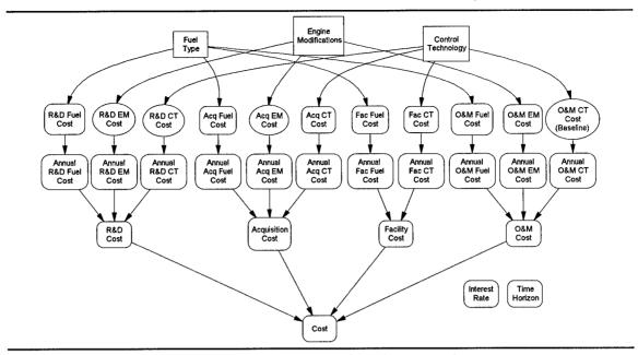
Figure 33 Cost Module with Chance Nodes
