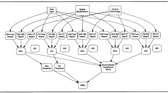
Figure 32 Environmental Compliance Module With Chance Nodes
