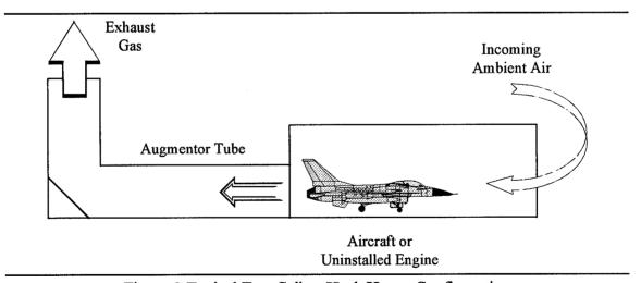
Figure 2 Typical Test Cell or Hush House Configuration
