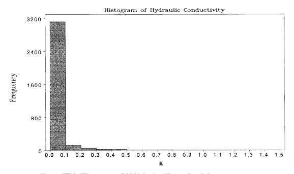
Figure III.3 Histogram of 3334 hydraulic conductivity measurements.
