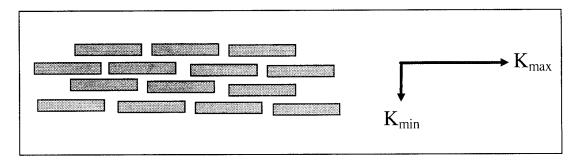
Figure II.9 Effect of grain orientation on hydraulic conductivity. (Adapted from lecture by Maj. Edward Heyse, 1995)
