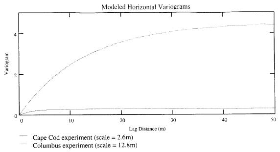
Figure II.5 Horizontal variograms from Cape Cod and Columbus AFB experiments.
