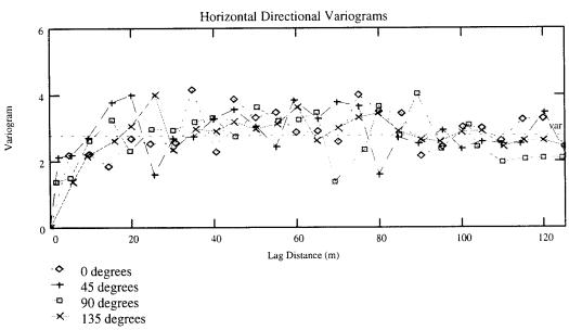
Figure III.7 Experimental horizontal directional variograms.
