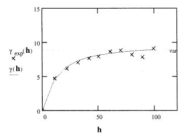
Figure II.4 Fitting a model variogram to an experimental variogram.
