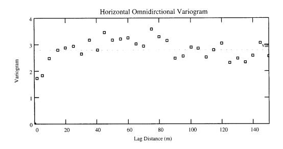
Figure III.9 Experimental horizontal omnidirectional variogram.
