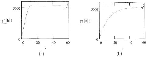
Figure II.3 (a) Spherical and (b) exponential variogram models.
