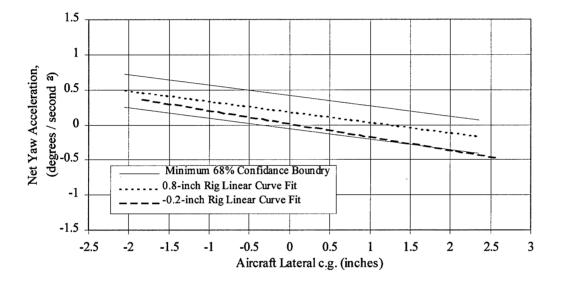
Figure 4-6. F-15B flight test effects of changing differential stabilator at 15,000 feet (4,572 meters) PA.
