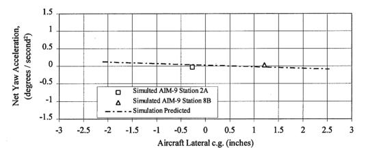
Figure 4-7. F-15 simulation net yaw acceleration predictions at 32,000 feet (9,754 meters) PA with 0.5-inch (12.7-millimeter) RLED and 0.5-inch (12.7-millimeter) LLEU.
