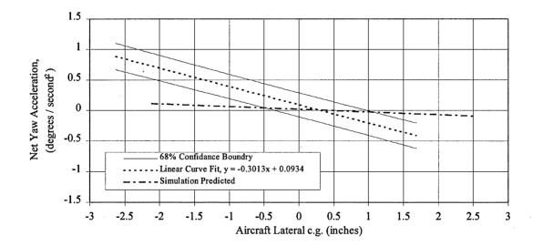
Figure 4-3. Simulation and flight test comparison of F-15 net yaw acceleration at 32,000 feet (9,754 meters) PA, with 0.4-inch (10.1-millimeter) RLED and 0.4-inch (10.1-millimeter) LLEU.
