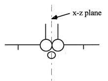
Figure 2-3. x-z plane of symmetry.
