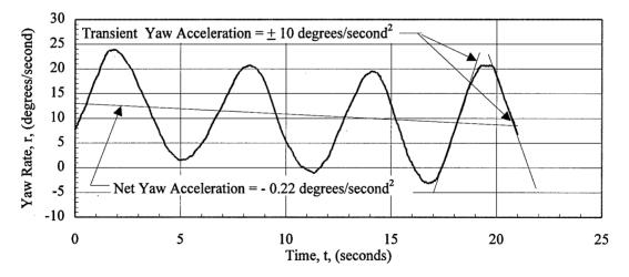
Figure 4-10. Transient yaw acceleration for sample flight test F-15B data.
