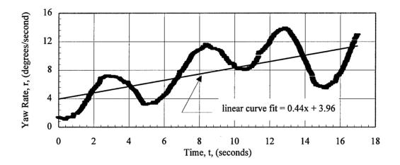
Figure 3-4. F-15B yaw rate at 32,000 feet (9,754 meters) PA for zero fuel asymmetry with 0.4 inch (10.1 millimeter) LLEU and 0.4 inch (10.1 millimeter) RLED.
