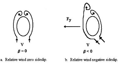
Figure 2-5. Forebody vortex flows over an aircraft nose shape at high AOA.
