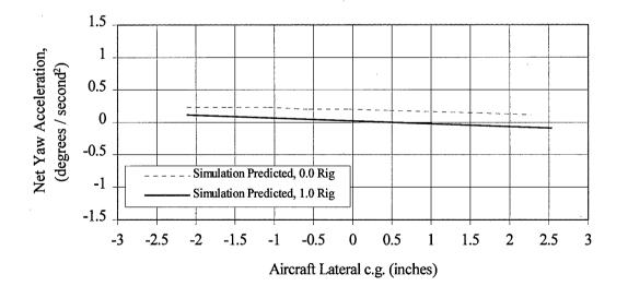
Figure 4-4. Simulator predicted effects of changing differential stabilator bias at 32,000 feet (9,754 meters) PA.
