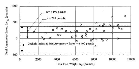
Figure 4-12. F-15B S/N 76-0130 lateral fuel asymmetry error, front cockpit indicator.
