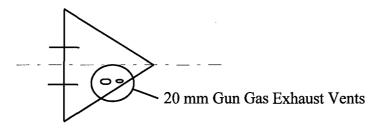
Figure 2-4. 20 mm gun gas exhaust vent location.
