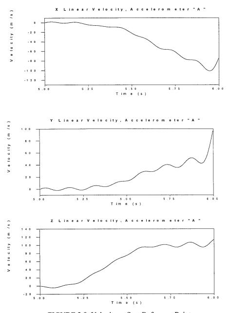
FIGURE 2.8 Velocity at Seat Reference Point
