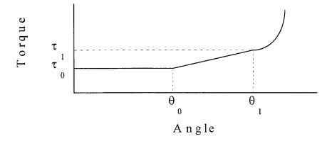
FIGURE 4.1 Modified Joint Resistive Torque Function
