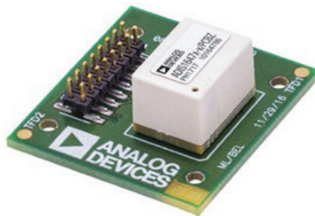
FIGURE 9 Analog Devices ADIS16470 MEMS IMU: The device footprint measures approximately 1.25'' \times 1.35'' .
