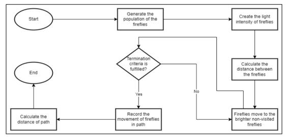
Fig. 2 - Flowchart of Firefly Algorithm (FA)
