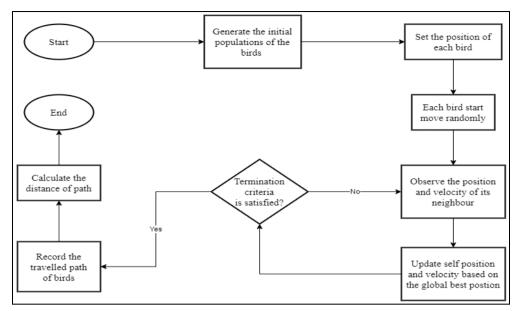
Fig. 1 - Flowchart for Particle Swarm Optimization (PSO)
