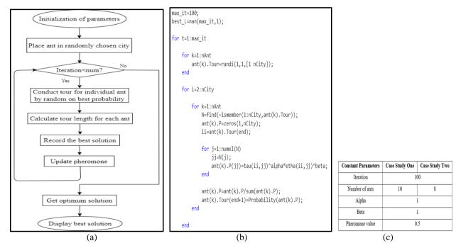
Fig. 4 - (a) ACO Algorithm; (b) ACO snippet code; (c) ACO initialization values
