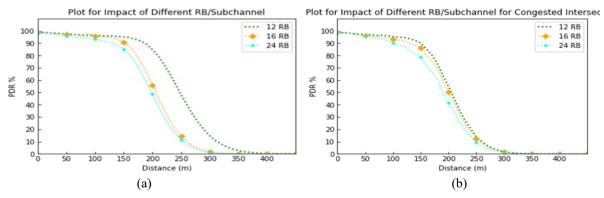
Fig. 5 - Impact of number of RB in (a) congested highway; (b) congested road intersection
