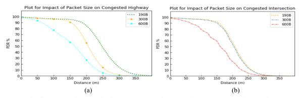
Fig. 6 - Impact of packet size in (a) congested highway; (b) congested Road intersection
