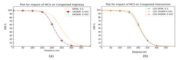
Fig. 4 - Impact of MCS in (a) congested highway; (b) congested road intersection
