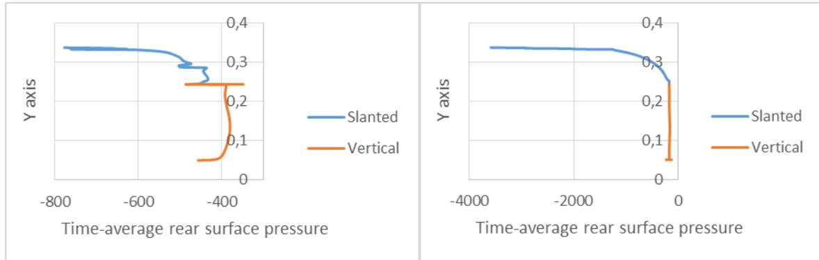
**Fig. 12 - Time-average surface pressure of rear end VS Y-axis graph with different Lb, (left) 120 (right) 200**
