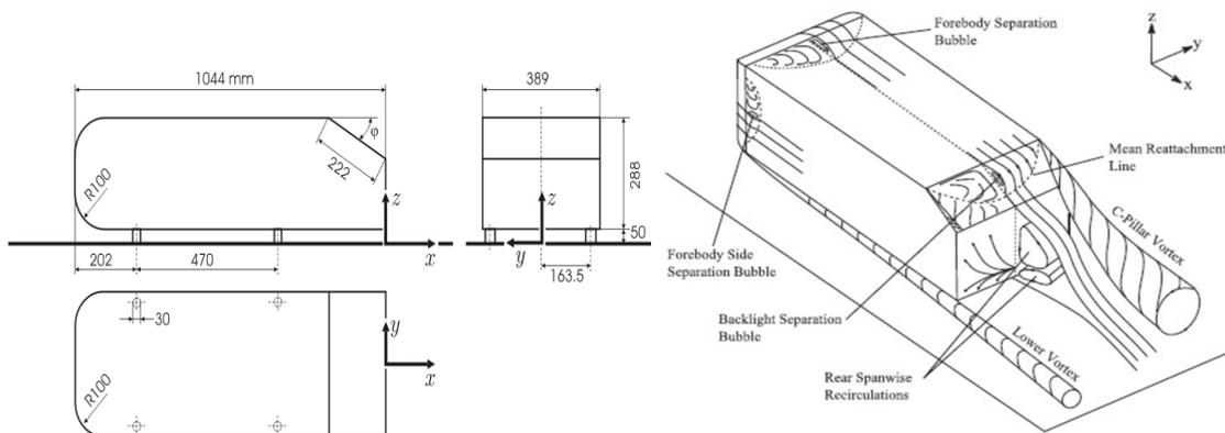
Fig. 1 - (a) Ahmed Body; (b) flow pattern on Ahmed Body model (Ahmed et al. 1984)
