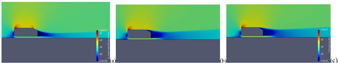
**Fig 10 - Time-average velocity contour with different  $L_a$  (a) 10; (b) 50; (c) 90**
