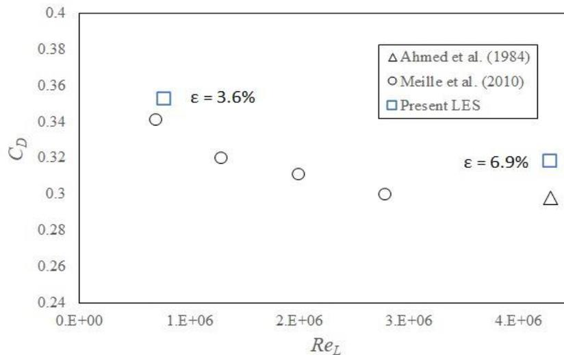
Fig. 5 - Time-averaged drag coefficient plotted against Reynolds number
