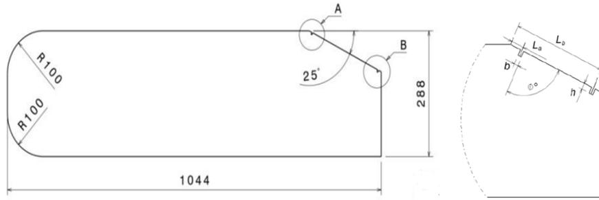
**Fig. 3 - Design of CFJ on Ahmed Body. Dimension in mm**
