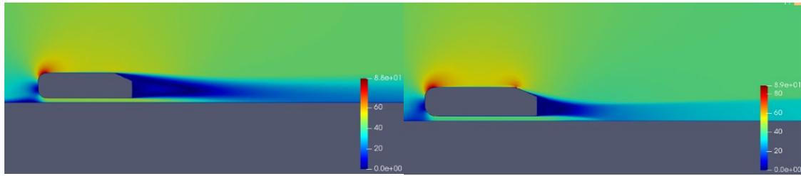
**Fig. 11 - Time-average velocity contour with different Lb, (left) 120 (right) 200**
