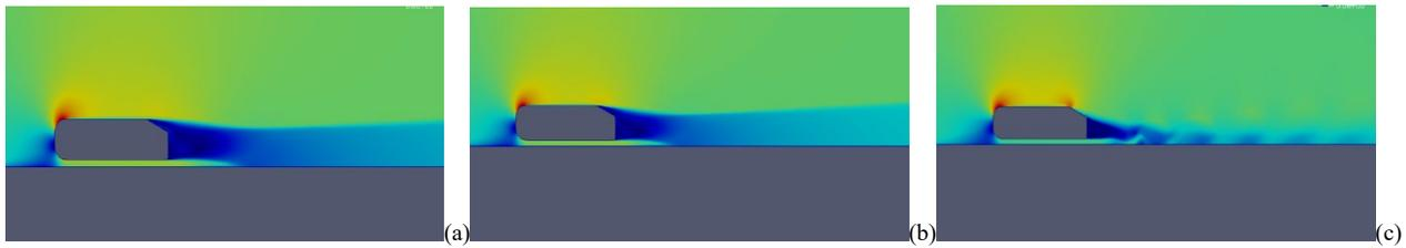
**Fig 9 - Instantaneous velocity contour of CFJ14 cases (a) 10m/s; (b) 25 m/s; (c) 40m/s**
