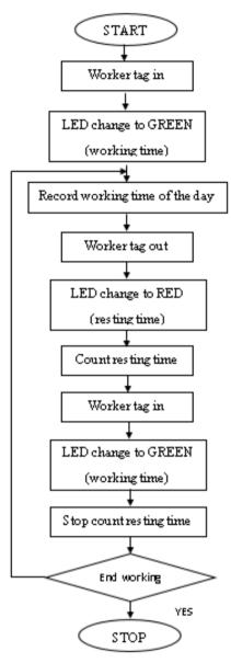
Fig. 2 - Flowchart of the monitoring system
