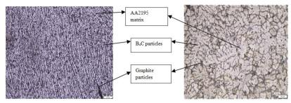
Fig. 3 - (a) Optical image of hot rolled sample after rolling AA2195-B4C-Gr composites; (b) optical image of casted sample before rolling AA2195-B4C-Gr composites
