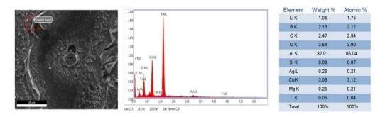
Fig. 4 - SEM EDAX Spectrum of the casted AA2195-B4C- Gr composites
