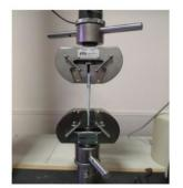
Fig. 14 - Tensile testing machine
