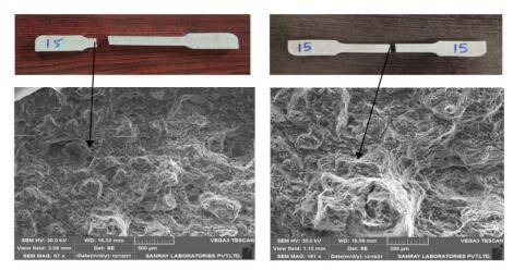
Fig. 19 - Casted AA2195-B4C-Gr MMCs and Hot Rolled HT AA2195-B4C-Gr MMCs and tensile fractured surfaces SEM images Casted & Hot Rolled aging AA2195-B4C-Graphite MMCs
