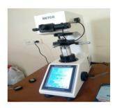
Fig. 11 - Vickers Micro hardness machine
