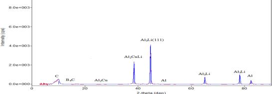
Fig. 7 - XRD pattern of the Hot rolling of AA2195-B4C- Gr composites
