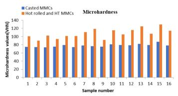
Fig. 12 - Micro hardness variation prior and later hot rolling process
