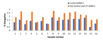
Fig. 18 - Variation of ductility before rolling and after hot rolling & HT MMCs
