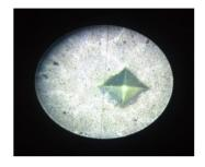
Fig. 9 - Vickers Micro hardness Diamond pyramid Indenter
