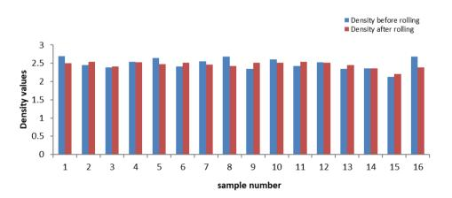
Fig. 21 - Density values before and after rolling of AA2195-B4C-Gr MMCs with sample number
