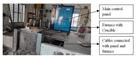
Fig. 1 - Medium frequency induction furnace
