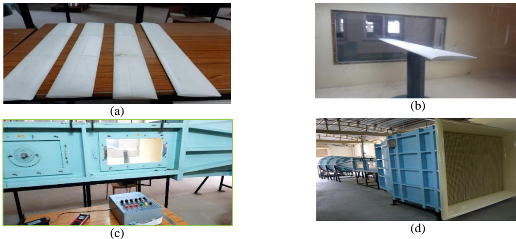
Fig. 3 - Wind tunnel set-up (a) 3D-printed models; (b) strain gauge balance platform; (c) 6-D component system; (d) LSWT
